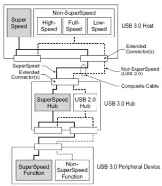
Note: Simultaneous operation of SuperSpeed and non-SuperSpeed modes is not allowed for peripheral devices.
