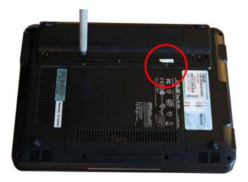
2. Locate the removable backplate on the bottom of the Eee PC. Unscrew the two retention screws.
