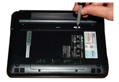
8. Snap the backplate back on, and screw in the two retention screws.
