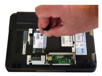
7. Screw in the retention screws to secure the SaberTooth SSD in place.
